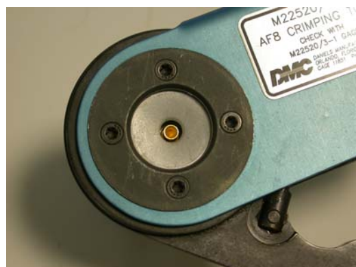
Fig. 10 crimping tool backside with socket
