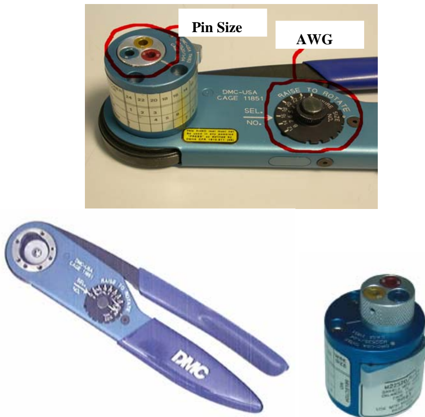
Fig.8 crimping tool M22520/1-01 and turret M22520/1-04
